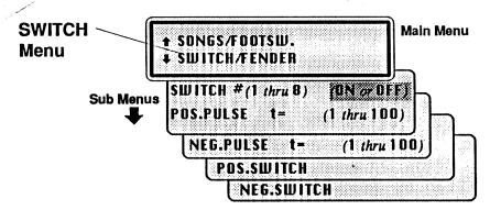
Because different devices utilize different kinds of footswitches, the MS-8 has been designed to cover a number of possibilities. Thus, each of the 8 SWITCHES can be set up to operate in 4 different modes:
