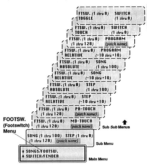
This sub menu actually has 10 sub *sub* menus. There are two ways to move between the 10 sub *sub* menus: 1) by using the Left and Right Menu Select buttons to move the cursor to the variable in the upper right corner, then using the +1/YES and -1/NO buttons to move up and down the sub *sub* menus; and 2) by using the F1 and F2 buttons to move up and down the sub *sub* menus.
