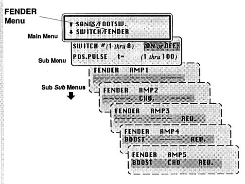
If you have one of the new Multiplexing Fender amplifiers (see chart in BACK PANEL section), you will use these sub *sub* menus to match the MS-8 with your specific model of amplifier. Simply use the +1/YES and -1/NO buttons to change the value of these sub *sub* menus until you get the one that matches the footswitch that came with your amplifier.
